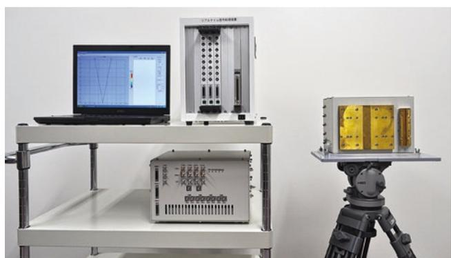
Stepped multiple-frequency CPC (Complementary Phase Code) millimeter-wave radar
