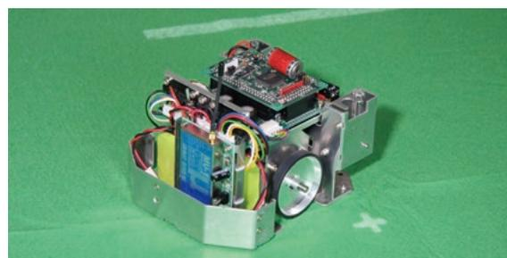
Robot conforming to the RoboCup Soccer Small Size League
