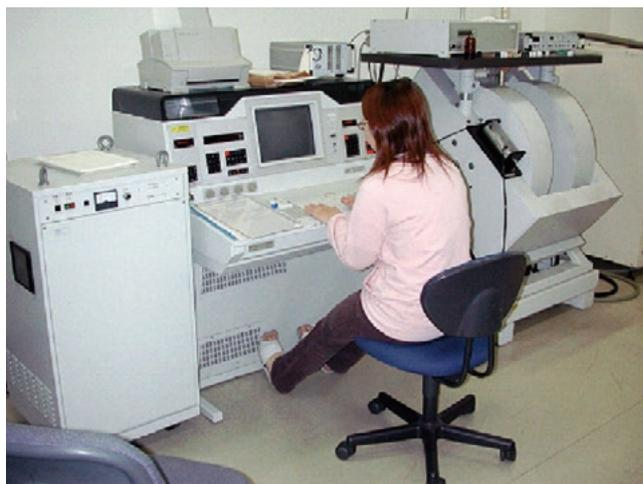
Electron spin resonance spectrometer
