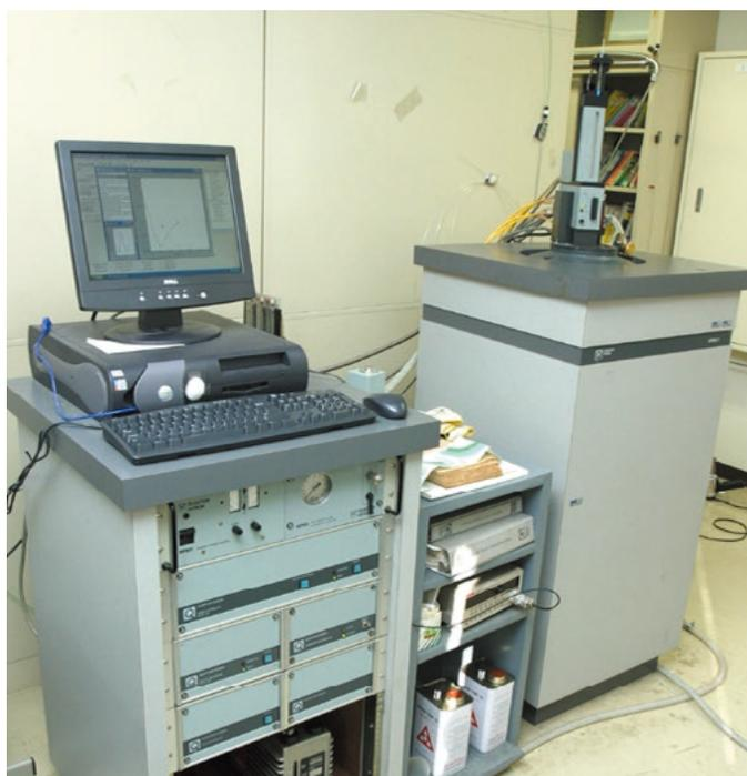
Superconducting quantum interference device magnetometer
